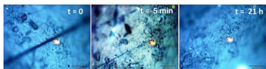
Figure 7. Optical micrographs of scratches of the network sample before ( t=0 ) and after healing at 60 °C for 5 min and 21h.
